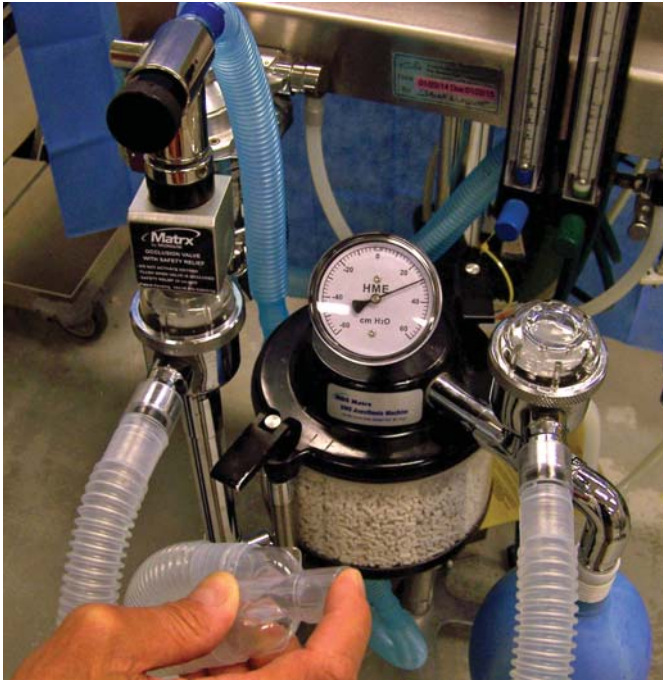
Figure 4.5 Pressure check of a circle rebreathing system. The pop-off valve is closed, the Y-piece occluded, and the O 2 flush valve is activated to distend the bag and develop a pressure equal to 30 cm H 2 O.
