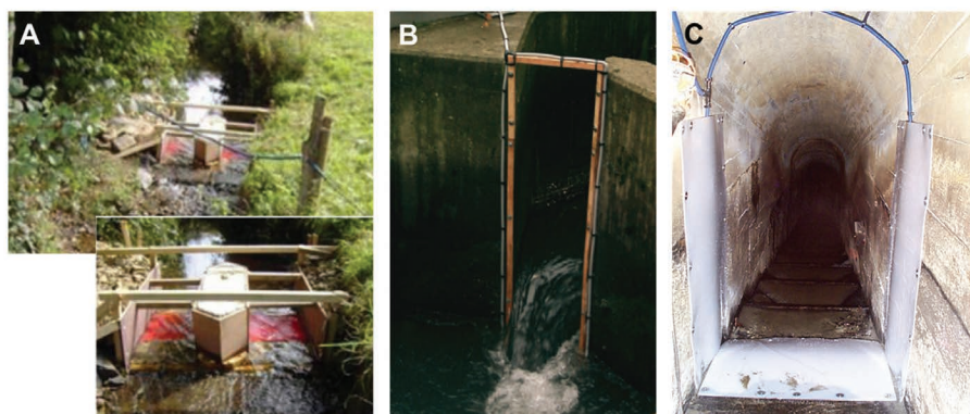
Figure 12.4. Passive tracking with fixed detection stations (antennas). Flatbed antennas in a small river, River La Roche, Normandy, France, FDX technology (© Irstea, M.L. Acolas, Inra experimentation site) (A). Swim-through antennas in a pool fish pass (B) and at a fish bypass entrance (C), HDX technology, River Gave de Pau, France (© Onema, P. Gomes).
